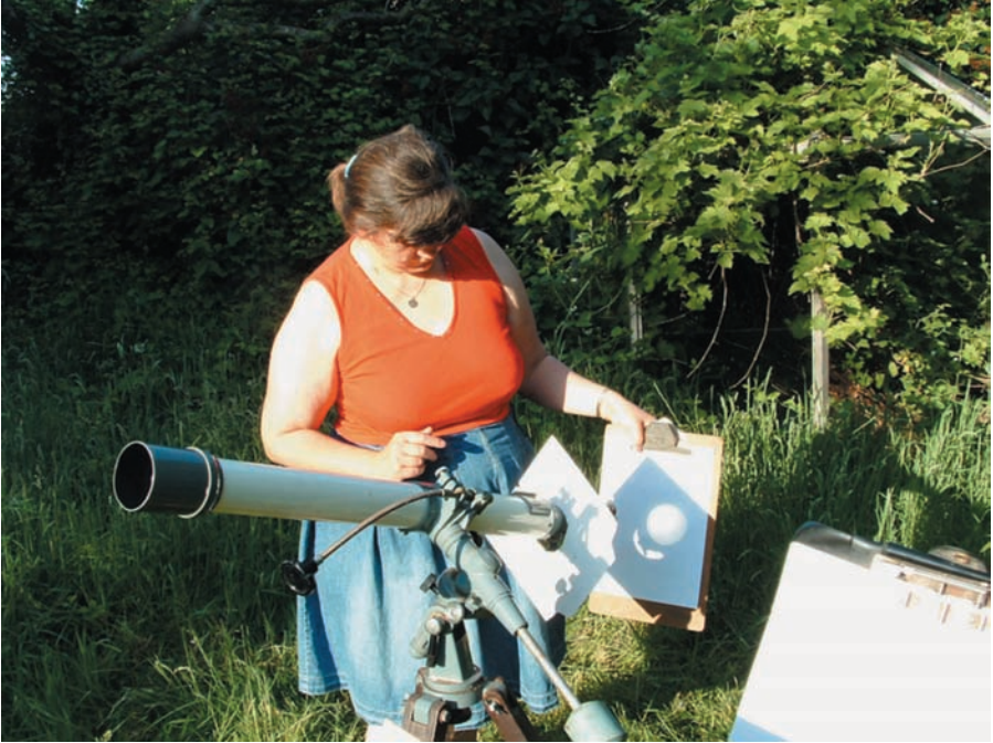
Figure 3.3. Projection through a small telescope is the simplest and safest way to observe sunspot activity.
